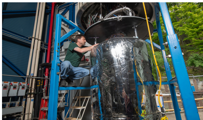
A tank is used in CryoFILL experiments to liquefy oxygen at minus 290 degrees Fahrenheit as it could be done on the Moon or Mars. The tests conducted at NASA's Glenn Research Center in Cleveland used Fiber Optic Sensing System (FOSS) developed by NASA's Armstrong Flight Research Center, in Edwards, California, to measure oxygen temperatures inside the tank. NASA/Bridget Caswell
