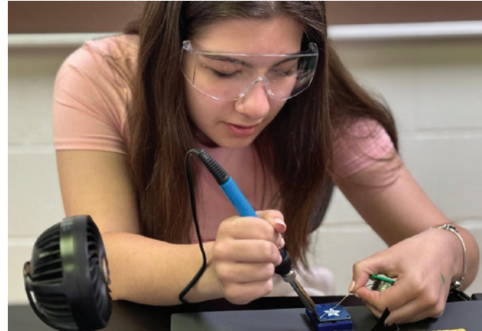
A NASA TechRise student team member focuses on soldering a microSD card breakout board component. Credit: Ashley Rowan
