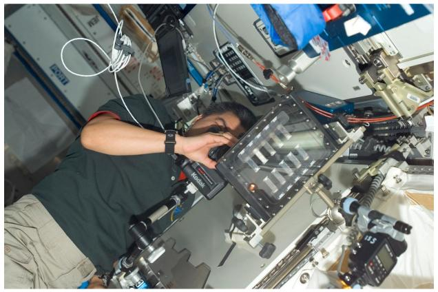
The Binary Colloidal Alloy Test-6, Phase Separation (BCAT-6, Phase Separation) experiments examine conditions that result in colloidal crystallization, melting, self-organization, and phase separation of colloidal systems. The evolution toward equilibrium through time is captured on the International Space Station (ISS) or with the accurate measurement of time frames correlated to the pictures taken by a new kind of automated camera.
