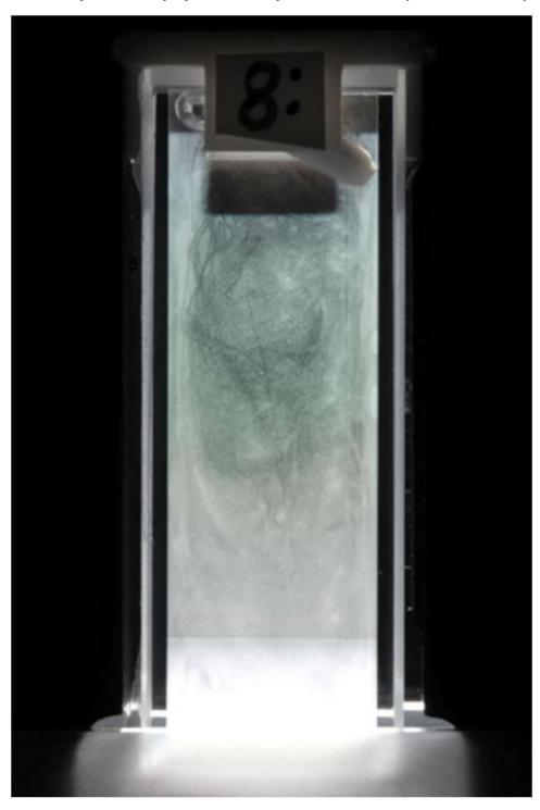
The Binary Colloidal Alloy Test 6: Polystyrene – Deoxyribonucleic Acid (BCAT-6-PS-DNA) uses DNA as a type of molecular glue to specifically stick small particles together. The experiment uses microscopic polymer beads in solution (colloids) that have been coated with DNA. The DNA only binds to its complement and hence keeps specific particles together to form designer crystals.
