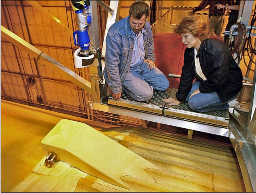
Figure 36. The bipod ramp of spray-on insulating foam that covers the attachment point of the bipod to the external tank. Compare this photo to Figure 37 below with no bipod ramp. (Figure I5 in Charles J. Camarda, "Space Shuttle Return-to-Flight Following the Columbia Tragedy." NATO Science and Technology Lecture Series on "Hypersonic Flight Testing," March 14, 2014).
