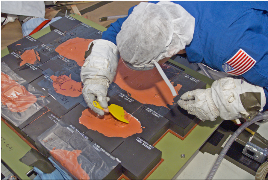
Figure 43. Onboard a KC-135 aircraft, astronaut Rex J. Walheim smooths and removes excess putty while rehearsing an EVA task for repairing damaged Shuttle tiles. The aircraft flew a series of special parabolas to practice the activity in free-fall. (NASA Image JSC2003-E-52340)
