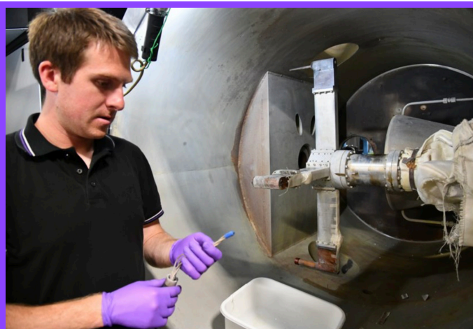
Christopher Naughton (Code TSA) installs one of the nose inlet test models in the CO 2 plasma jet chamber at the University of Illinois Urbana-Champaign CHES facility. Credit: NASA
