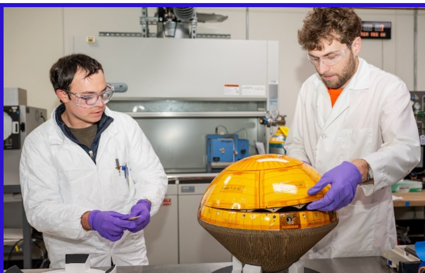
Eli Hiss (left) and Bohdan Wesely (right), associate with the Thermal Protection Materials Branch at NASA Ames, holding the HEEET seamless, single-layer heatshield for Rocket Lab’s Venus mission.
