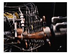
**RCL-11 Instrumented Chamber for 25-lbf Nozzle Study**
