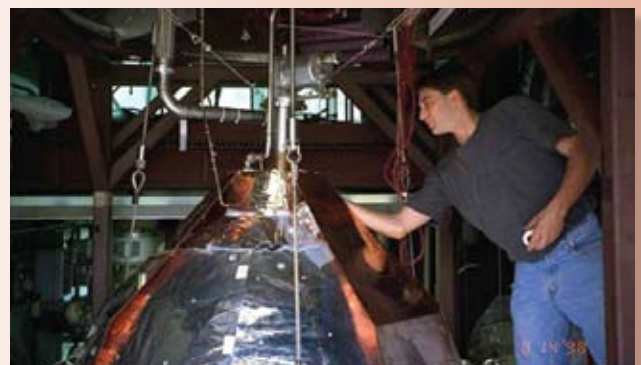
Cryocooler preparation for zero boiloff test (SMiRF)
