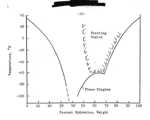
Starting fuels which are miscible with gasoline do not behave in the same way, and this suggests that a separate ignitor chamber directing a flame into the combustion chamber would be more reliable and would permit attainment of satisfactory starts at  $-76^{\circ}F$  or below.
