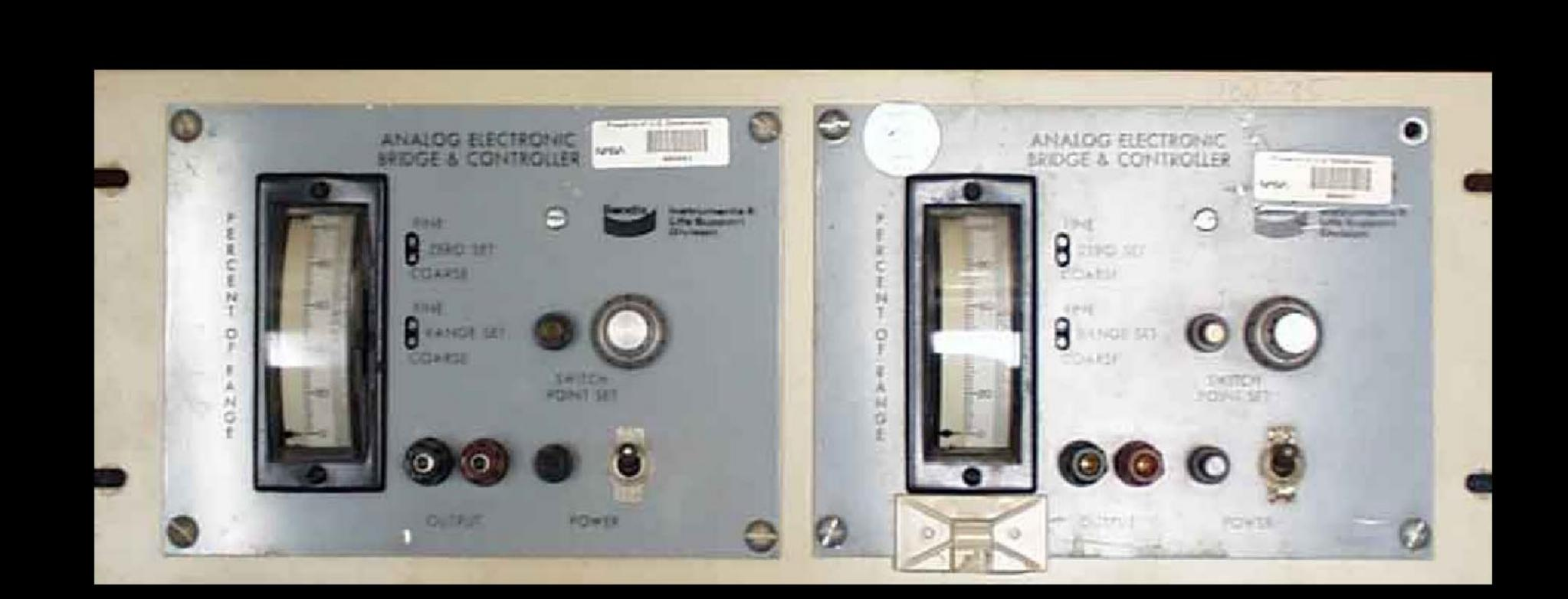
This is a ramp generator panel. According to former RETF Engineer Doug Bewley, "These ramp-generators were used to provide reference electrical signals to the controllers who then positioned the valves that provided the liquid oxygen and liquid hydrogen to the rocket engine being tested."
