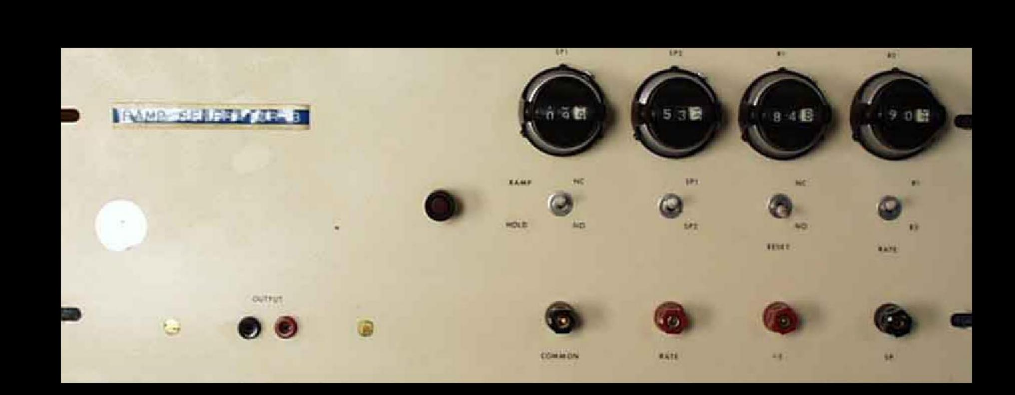
This panel and electronic equipment controlled the speed at which the valves were opened to allow the fuel and oxidizers into the test cell.
