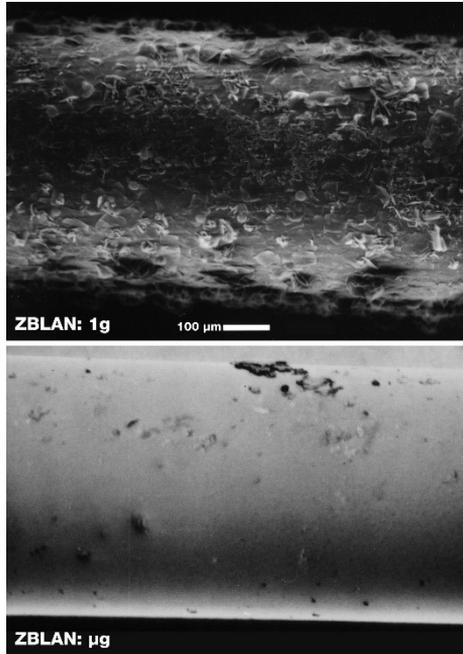
*Figure 14. Scanning electron microscope (SEM) images of the surface of ZBLAN fibers pulled in microgravity (bottom) and in 1g during a typical ground-based manufacturing process (top). The crystallization and defects that occur during ground-based manufacturing result in scattering of the optical signal, significantly degrading the quality of the fiber. Image credit: NASA*
