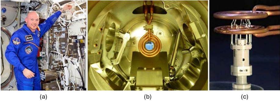
*Figure 5. (a) ESA astronaut Alexander Gerst is shown installing the ISS-EML facility (photo courtesy of ESA), (b) levitation coils within the processing chamber (photo courtesy of Airbus), and (c) wire cage sample holder used to keep the sample within the coil center. Photo courtesy of Airbus.*
