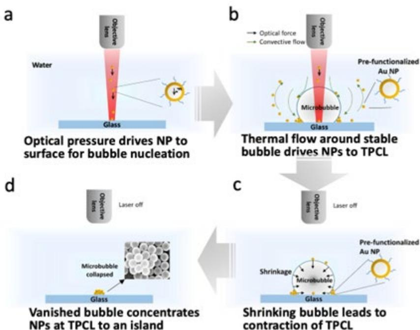
Figure 17. Schematics of (a) optical pressure force driving suspended NPs to the surface; (b) laser-generated photothermal bubble and the flow surrounding it drives suspended NPs to the three-phase contact line (TPCL); (c) laser turned off to allow bubble shrinking, which leads to TPCL contraction; and (d) concentrated NP island deposited by SSBD due to the complete contraction of TPCL as the bubble vanishes. Inset in (d) is a representative scanning electron microscopy image of the SSBD spot.
