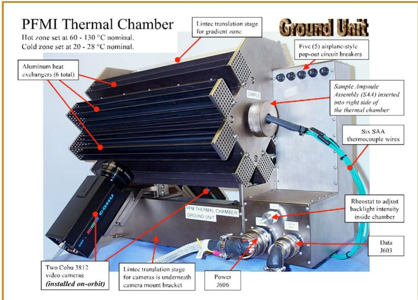
Figure 3. Labeled photo of the PFMI ground hardware. Image credit: NASA
