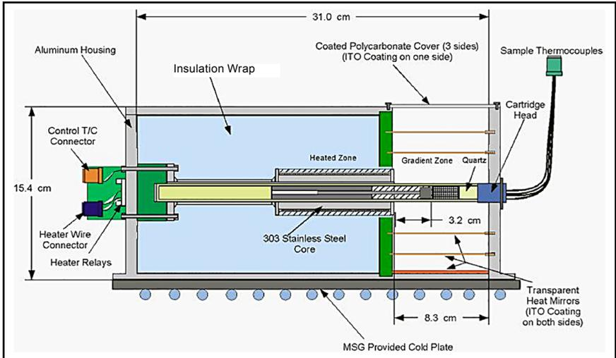
Figure 2. Cross-section of the SUBSA furnace. The sample is immediately to the left of the quartz plug. The baffle assembly is to the left of the sample. Image credit: NASA
