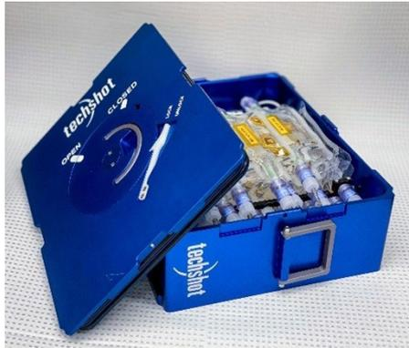
Figure 8. Photo of a Techshot fluid processing cassette designed for installation in the ADvanced Space Experiment Processor (ADSEP). Image credit: NASA
