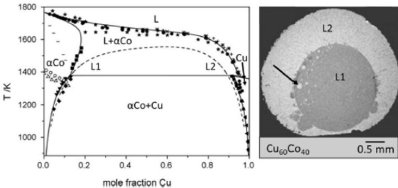
Figure 16. Miscibility gap in the Co-Cu system. (a) The binary phase diagram with thermodynamic predictions on phase composition (lines) and experimental verification (points). (b) Backscatter scanning electron microscope image of a levitated sample showing solidification following phase separation of two liquids with the arrow showing small, entrained droplets of Cu-rich liquid within the darker Co-rich second phase.
