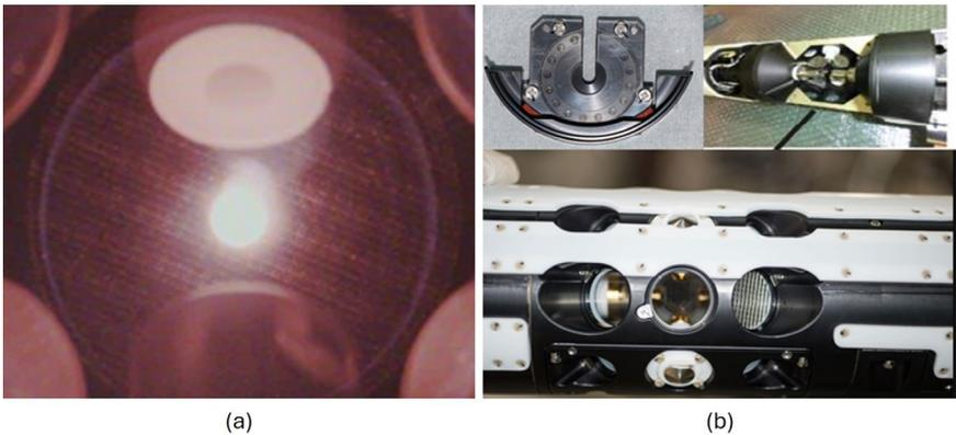
*Figure 4. (a) Molten metal oxide sample levitated in the ELF and (b) Sample cartridge and sample holder for material processing. Image credit: NASA*
