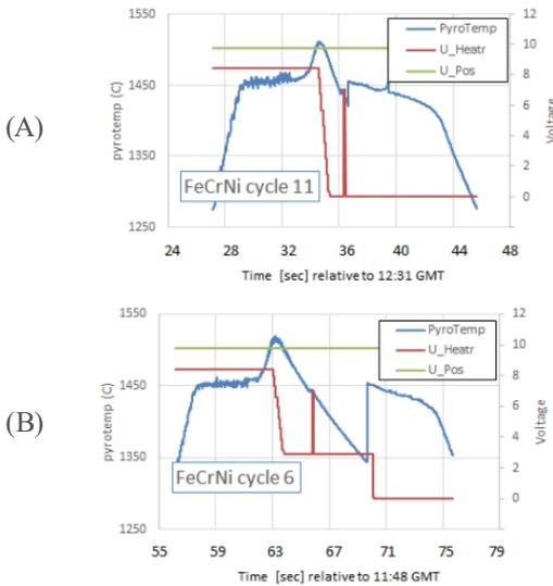
Figure 21 . Thermal profile from a ternary stainless steel alloy showing temperature (blue) resulting from applied positioner (green) and heater (red) EM fields from two different runs: (a) heater voltage goes to 0V to access laminar flow and (b) heater voltage is set to 3V to access turbulent flow. The heater pulse during the liquid cooling process is used to obtain thermophysical properties. Figure reproduced from Matson et al., 2016.
