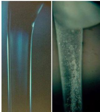
*Figure 13. Sections of ZBLAN fiber pulled during a microgravity parabolic flight (left) and during ground-based 1g manufacturing process (right). The rough surface/defects seen in the 1g manufactured fiber would greatly degrade the quality of the fiber by scattering the optical signal. Image credit: NASA/Marshall Space Flight Center*
