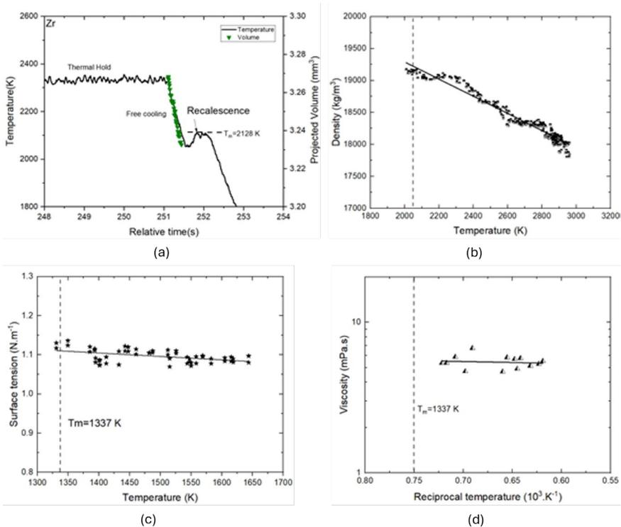
Figure 20. Data from microgravity Electrostatic Levitation at ISS-ESL processing; (a) A typical processing thermal cycle, (b) Density of Liquid Platinum, (c) Surface tension of liquid Au, and (d) Viscosity of liquid Au. Image credit: Dr. Douglas Matson
