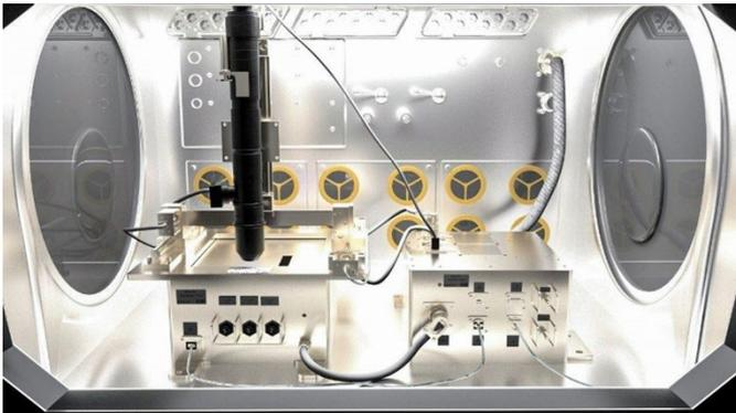
*Figure 12. A preflight image of the Microgravity Research for Versatile Investigations - Phase Change in Mixtures (MaRVIn-PCIM) system as it will be housed in the MSG.
