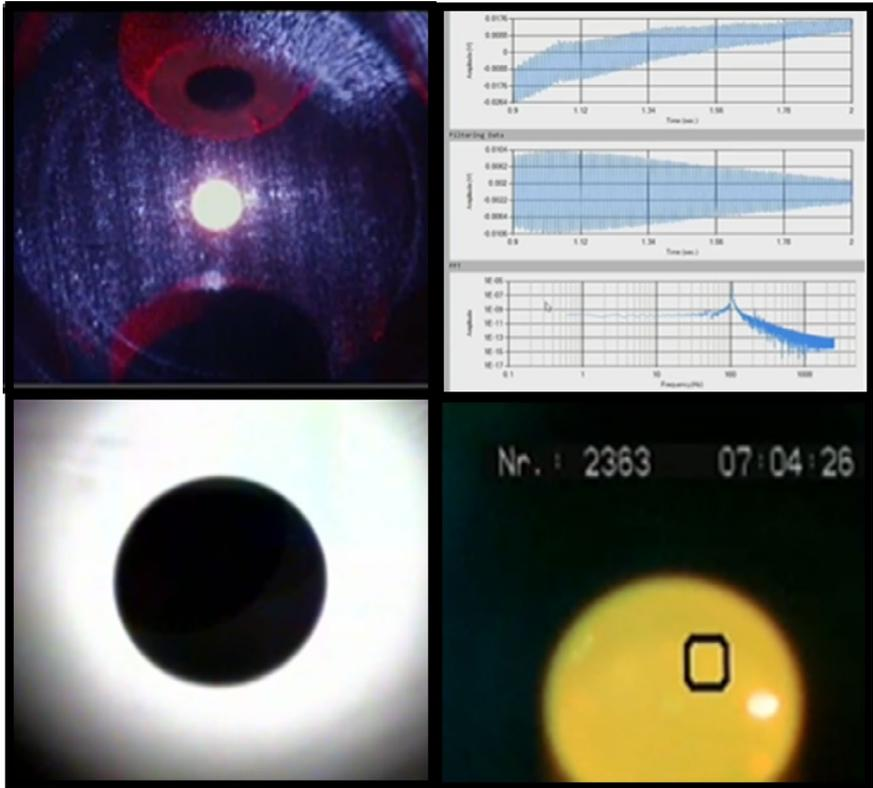
Figure 19. A molten Au sample levitated on the ISS-ELF (top left), induced surface oscillation signals (top right), backlit sample (bottom left), and pyrometer (bottom right).
