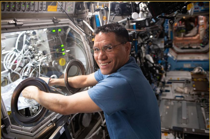
*NASA astronaut and Expedition 69 Flight Engineer Frank Rubio works in the Microgravity Science Glovebox (MSG) swapping graphene aerogel samples for a space manufacturing study. The physics investigation seeks to produce a superior, uniform material structure benefitting power storage, environmental protection, and chemical sensing. Photo courtesy of NASA.*
