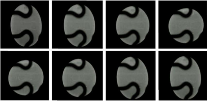
*Figure 18. A mosaic of frames showing selected side-view images at 30 kHz to demonstrate how a levitated sample deforms after pulse oscillation surface excitation. Figure reproduced from Matson et al., 2016.*
