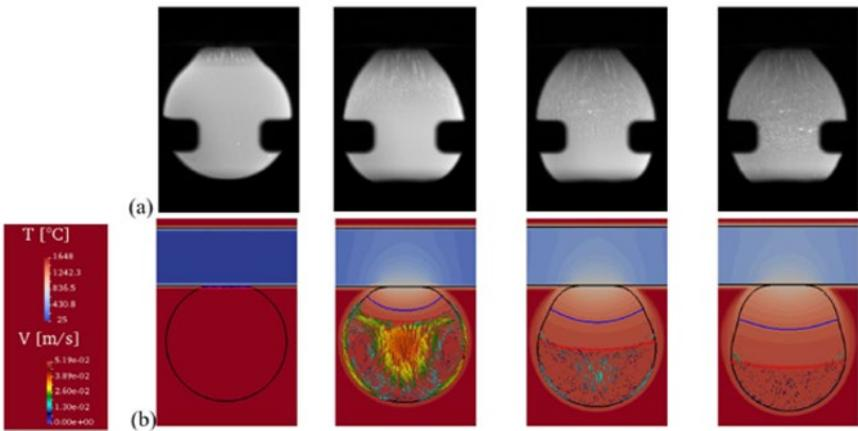
Figure 15. Evolution of structure during chill casting showing (a) a sequence of images of a Fe-0.9C-0.2Si steel solidifying in microgravity and (b) modeling of the dynamics and thermal history of the resulting solidification front.
