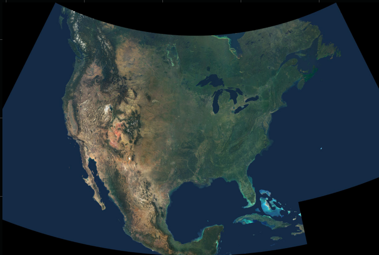
▲ This natural-color image combines cloud-free data from over 500 Multi-angle Imaging SpectroRadiometer orbits with shaded relief Digital Terrain Elevation models from the Shuttle Radar Topography Mission and other sources.
