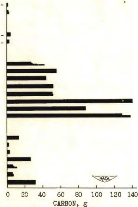
Effect of 50-percent evaporated temperature and fuel hydrocarbon type on carbon deposition.
