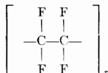
(2) FEP characteristics: Fluorinated ethylene propylene (FEP) tends to be more translucent (than TFE) at ambient conditions. It does not sublime like TFE, but becomes a very viscous fluid above a 500° to 530° F range. In addition, the material adheres to itself above this melting point range. The structure of the material is
