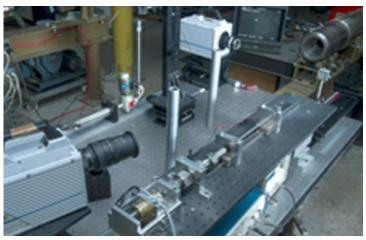
The microballistic powder gun has target heating capability and excellent impact accuracy at consistent velocities.
