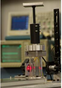
The ITF 'rain gun' is the only hydrometeor impact gun in the United States that can provide single impact performance data with known water-drop sizes.
