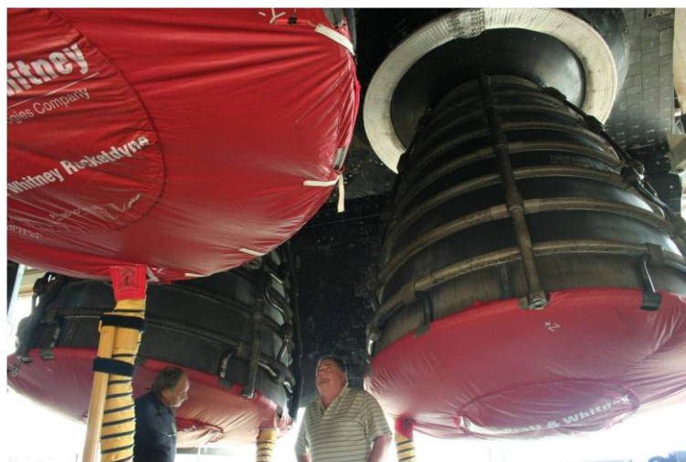
Figure 5.3.1-1. SSME Engines with Nozzle Closures and Purge Air Ducts Attached
