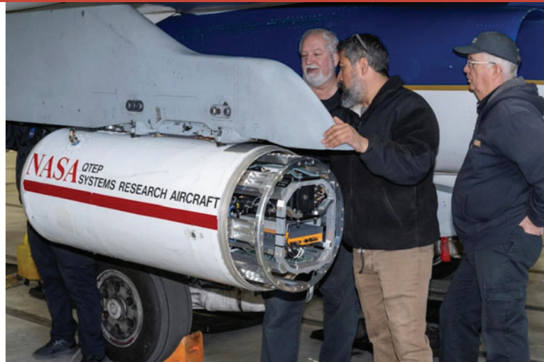
NASA engineers and technicians install Psionic's NDL system into a testing pod on a NASA F/A-18 research aircraft ahead of February 2025 flight tests at NASA's Armstrong Flight Research Center in Edwards, California. Credit: NASA
