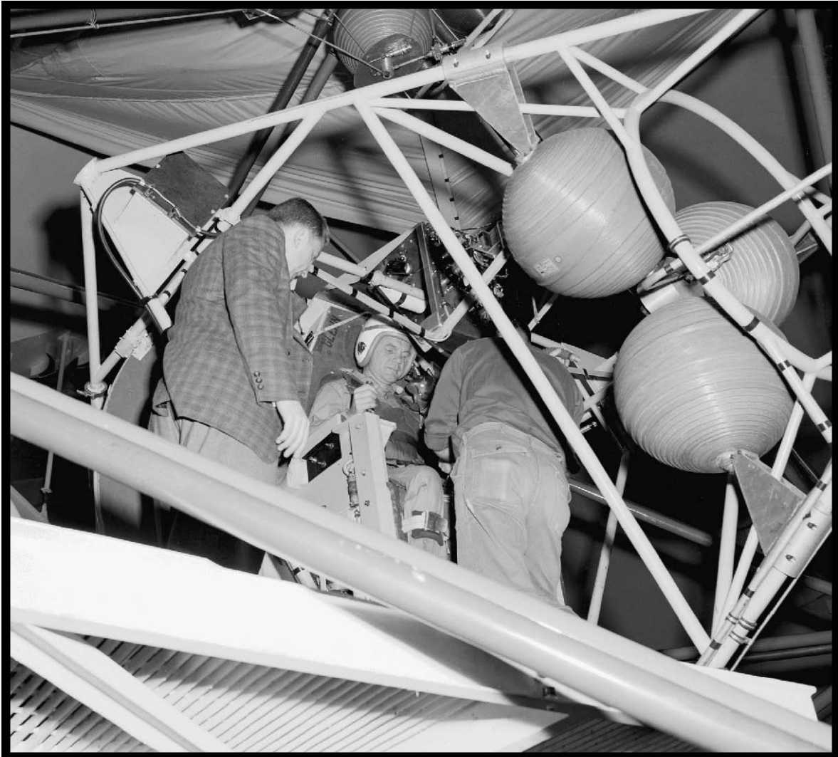
Figure 26.—John Glenn prepares for a test in the Multiple Axis Space Test Inertia Facility (MASTIF) inside of the AWT, 1960 (OH_Cuyahoga_Space-Power-Chambers_026).
