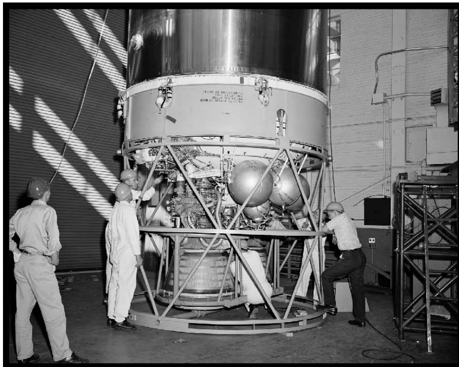
Figure 32.—Centaur 6A being inspected in the SPC shop area prior to insertion into the chamber, 1963 (OH_Cuyahoga_Space-Power-Chambers_032).
