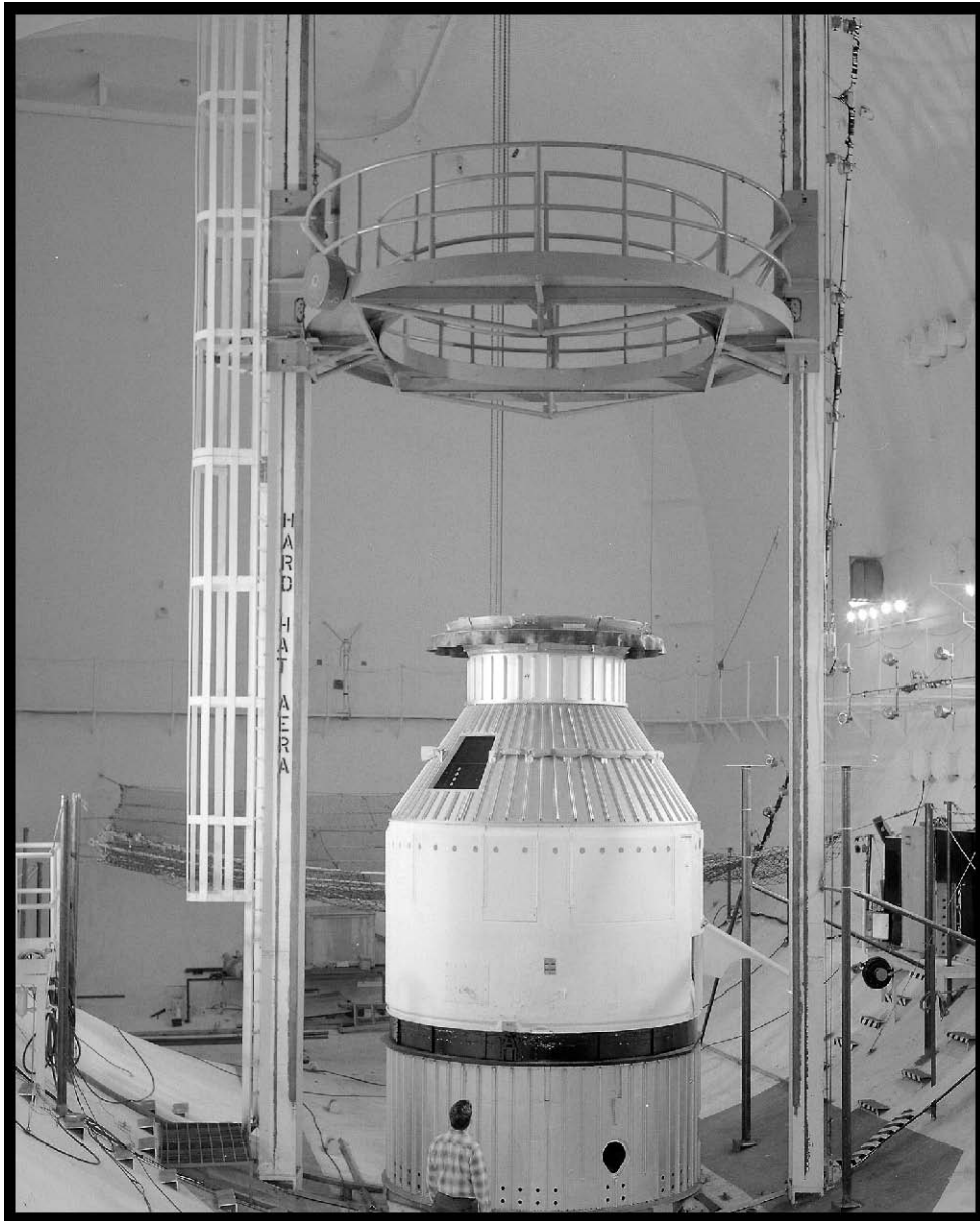
Figure 88.—Platform elevator in SPC No. 2 lifted above Centaur model (viewed from the north), 1968 (OH_Cuyahoga_Space-Power-Chambers_088).
