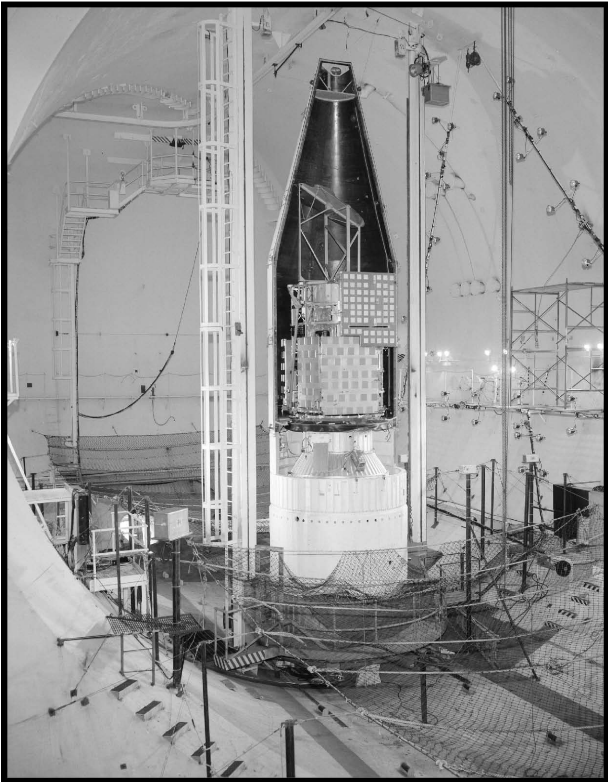
Figure 38.—Redesigned single-piece shroud being tested in SPC No. 2 for use on the OAO-C mission, 1972 (OH_Cuyahoga_Space-Power-Chambers_038).
