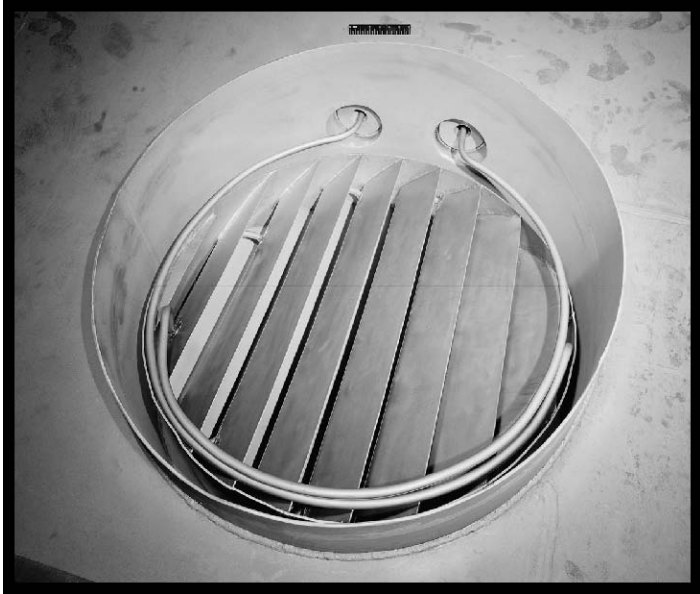
Figure 58.—Close-up of one of ten diffusion pump openings in the floor of SPC No. 1, 1962 (OH_Cuyahoga_Space-Power-Chambers_058).
