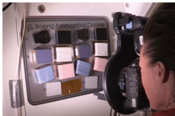
Touch panels installed for the ISS Boeing Antimicrobial Coating investigation.
