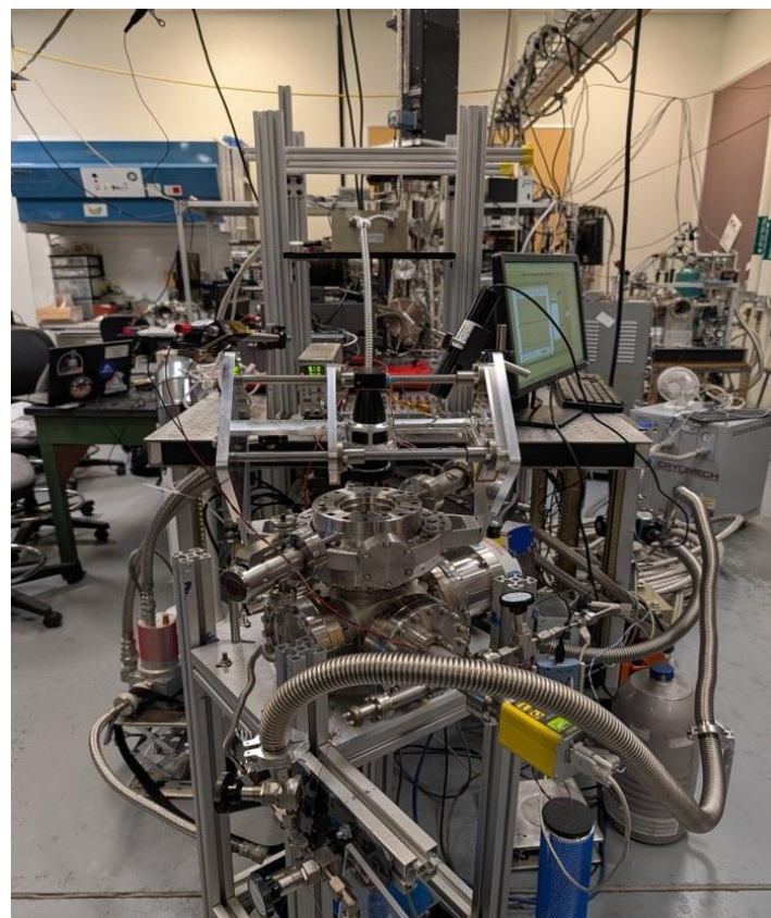
Figure 2. Low-temperature ice vacuum chamber equipped with vapor deposition and liquid aerosol injection to simulate samples on lunar surfaces and cryovolcanism on outer solar system bodies such as Europa and Enceladus.
