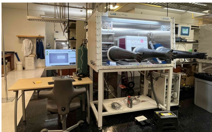
The nanoindentation system is housed within a glove box system that maintains less than 0.5 ppm of H 2 O and O 2 .
