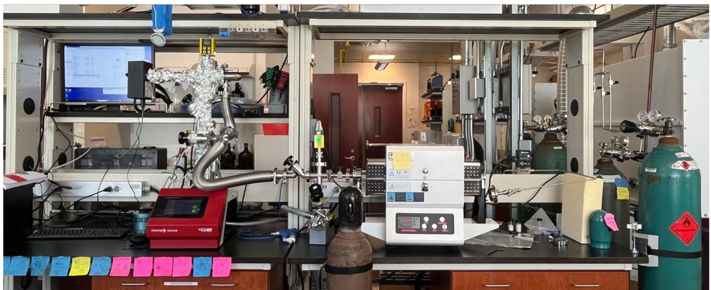
The thermal property characterization bench: a home-built dynamic vacuum furnace and vapor sorption system at UT San Antonio.
