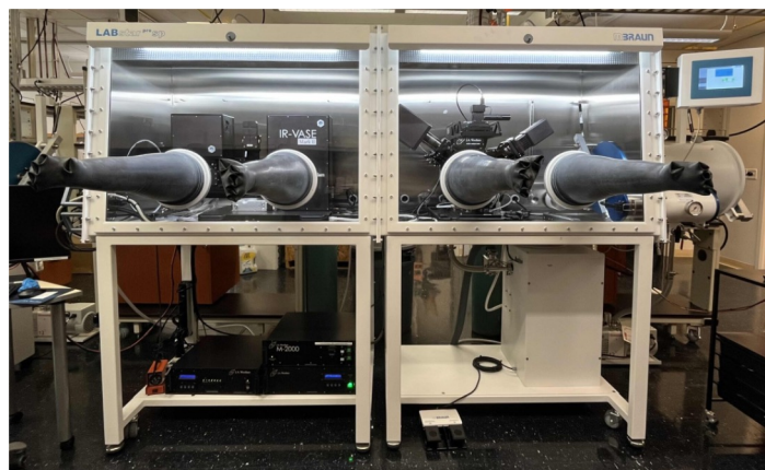
The dual-ellipsometry system is housed within a glovebox system that maintains less than 0.5 ppm of \text{H}_2\text{O} and \text{O}_2 .
