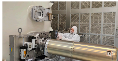
Marshall Grazing Incidence X-ray Spectrometer (MaGIX-2) testing in Stray Light Test Facility.
