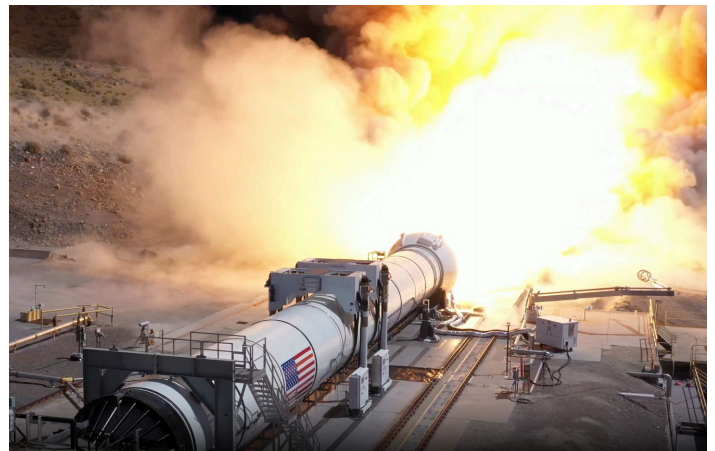
Five Segment Solid Motor Hot Fire Test.
