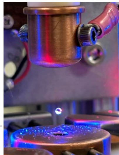
A liquid droplet levitating in the aqueous levitator
