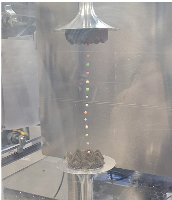
Styrofoam levitating between the transducers of the acoustic levitator. Sound waves create nodes that the material floats in.
