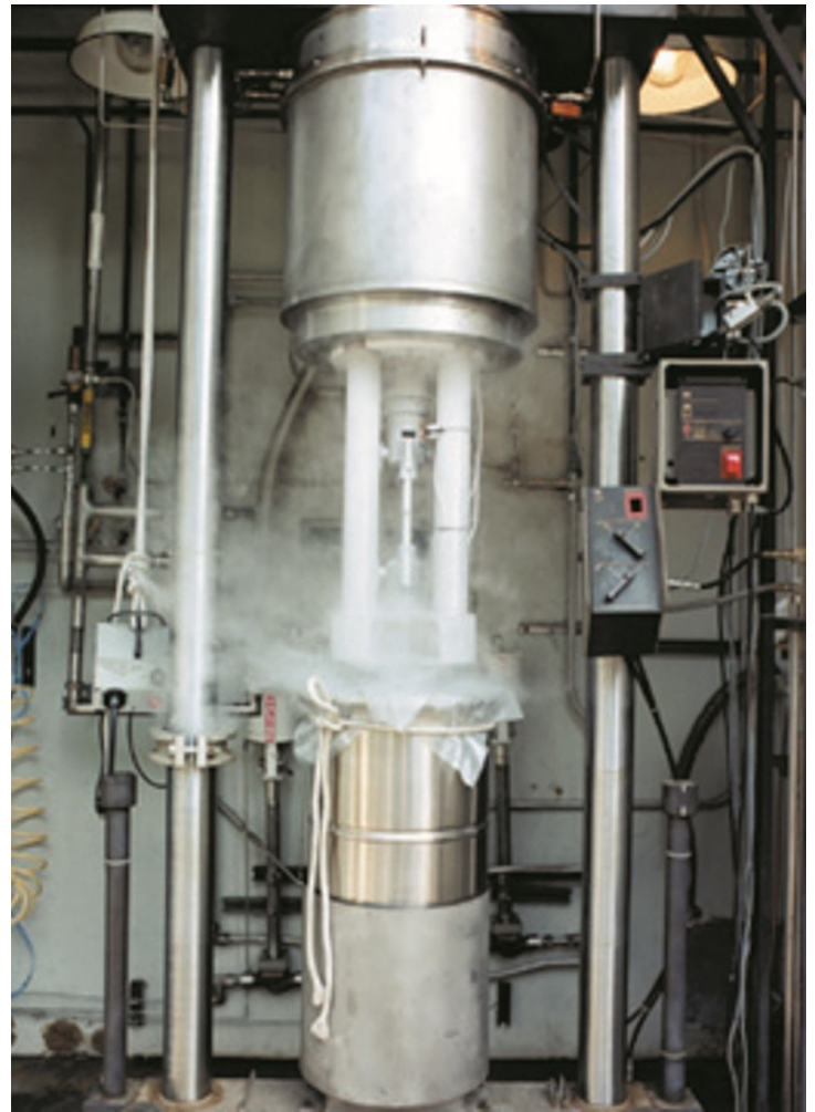
Tension Test Specimen in Liquid Hydrogen.
