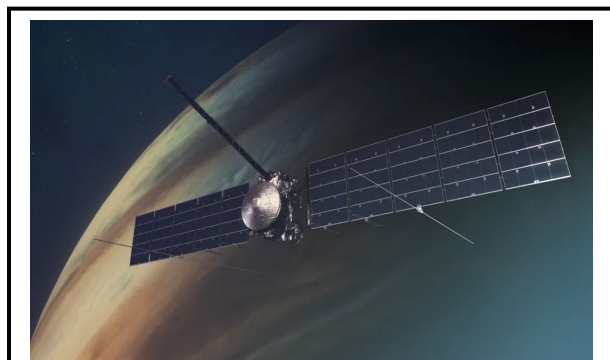
This artist's concept depicts NASA's Europa Clipper spacecraft with solar arrays fully deployed in orbit around Jupiter. Europa Clipper's solar arrays are the biggest NASA has ever developed for a planetary mission.
