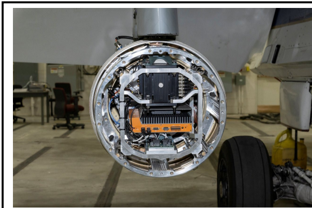
The Psionic Space Navigation Doppler Lidar (PSNDL) system installed in a testing pod on a NASA F/A-18 research aircraft ahead of February 2025 flight tests at NASA's Armstrong Flight Research Center in Edwards, California is shown here.
