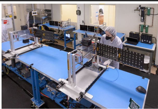
An engineer pictured at NASA's ARC inspects four spacecraft after completion of a solar array deployment test in preparation for the Starling demonstration.
