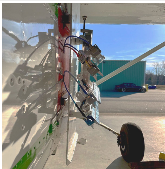
The Snow Water-equivalent Wide Swath Interferometer and Scatterometer (SNOWWI) instrument, developed under an IIP-21 award to the University of Massachusetts, Amherst, embarked on two sets of demonstration flights over Grand Mesa, CO, in January and March 2024, onboard a Cessna 208. SNOWWI is a new two-frequency, dual-polarized (VV & HV) Ku-band InSAR and scatterometer airborne instrument intended to measure and map snow properties – depth, density, height, and snow water equivalent (SWE) – over an extended region. These measurements are particularly important for water resources management and agriculture. (Image credit: P. Siqueira)
