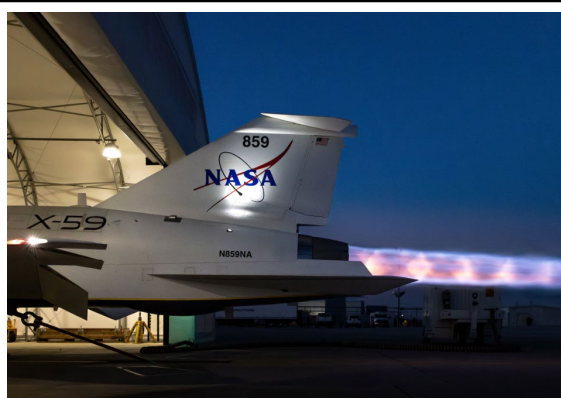
NASA's X-59 lights up the night sky with its Mach-diamond-infused flames during maximum afterburner testing at Lockheed Martin Skunk Works in Palmdale, California. The early 2025 test demonstrated the engine's ability to generate the thrust required for supersonic flight in support of NASA's Quesst mission.
