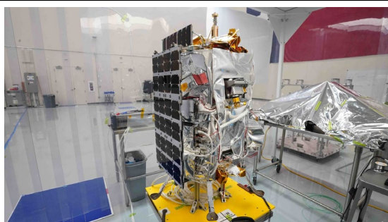
Intuitive Machines' IM-2 Micro-Nova Hopper, shown here, is a miniature Nova-C lander designed to search for water ice in permanently shaded regions of the moon. Credit: Intuitive Machines
