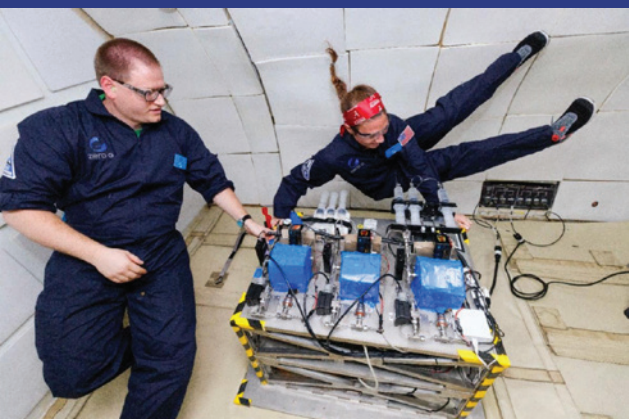
Bill Doig (left) and Brianna Warrenfeltz (right) operating the Teledyne EDR fuel cell water separator experiment during a reduced-gravity parabola on the first day of testing. Credit: Zero Gravity Corporation
