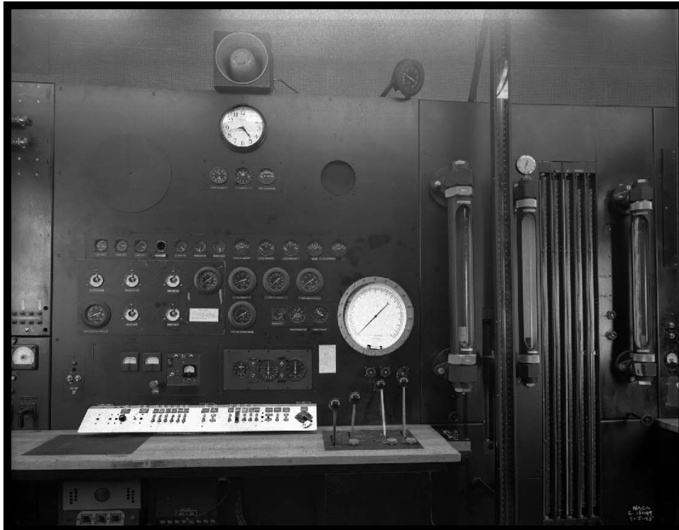
Figure 117.—Main console in the AWT control room, which was used control the engine in the test section, 1945 (OH_Cuyahoga_Altitude-Wind-Tunnel_118).
