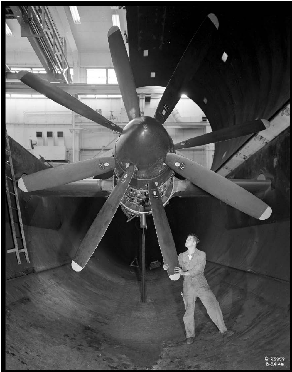
Figure 107.—The AWT test section was designed to be large enough to operate large reciprocating engines, 1949 (OH_Cuyahoga_Altitude-Wind-Tunnel_108).
