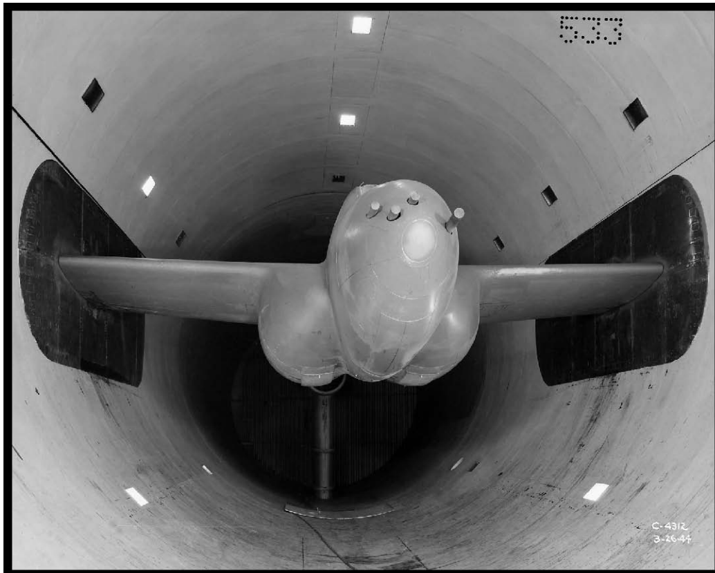
Figure 29.—Bell YP-59A Airacomet installed in the AWT test section, 1944 (OH_Cuyahoga_Altitude-Wind-Tunnel_030).
