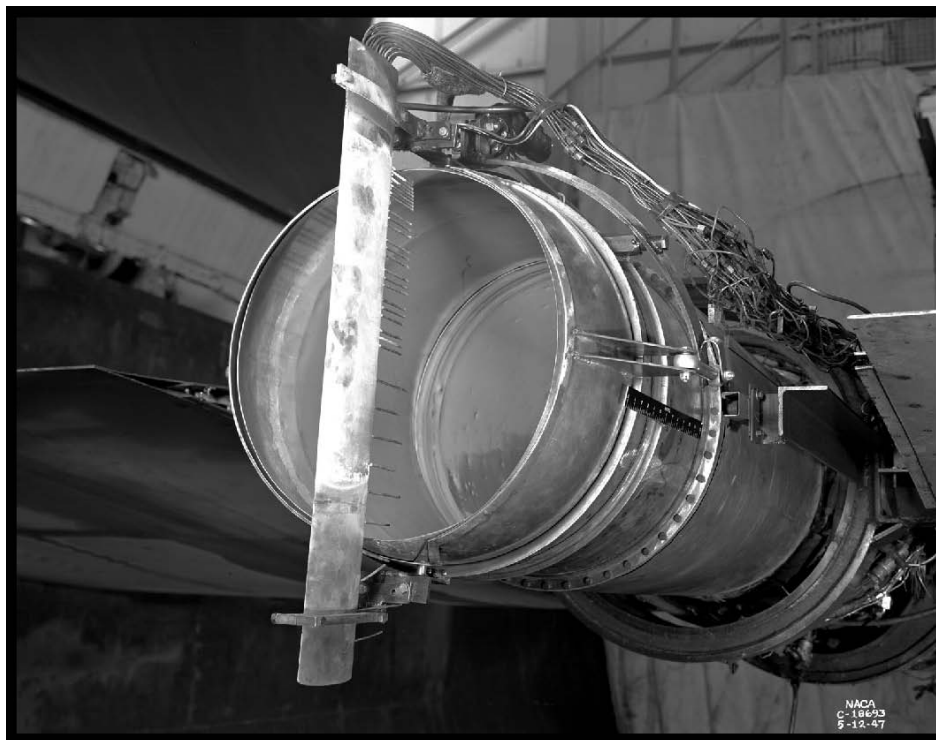
Figure 111.—Survey rake installed over the exhaust pipe of the Westinghouse 24C engine, 1947 (OH_Cuyahoga_Altitude-Wind-Tunnel_112).
