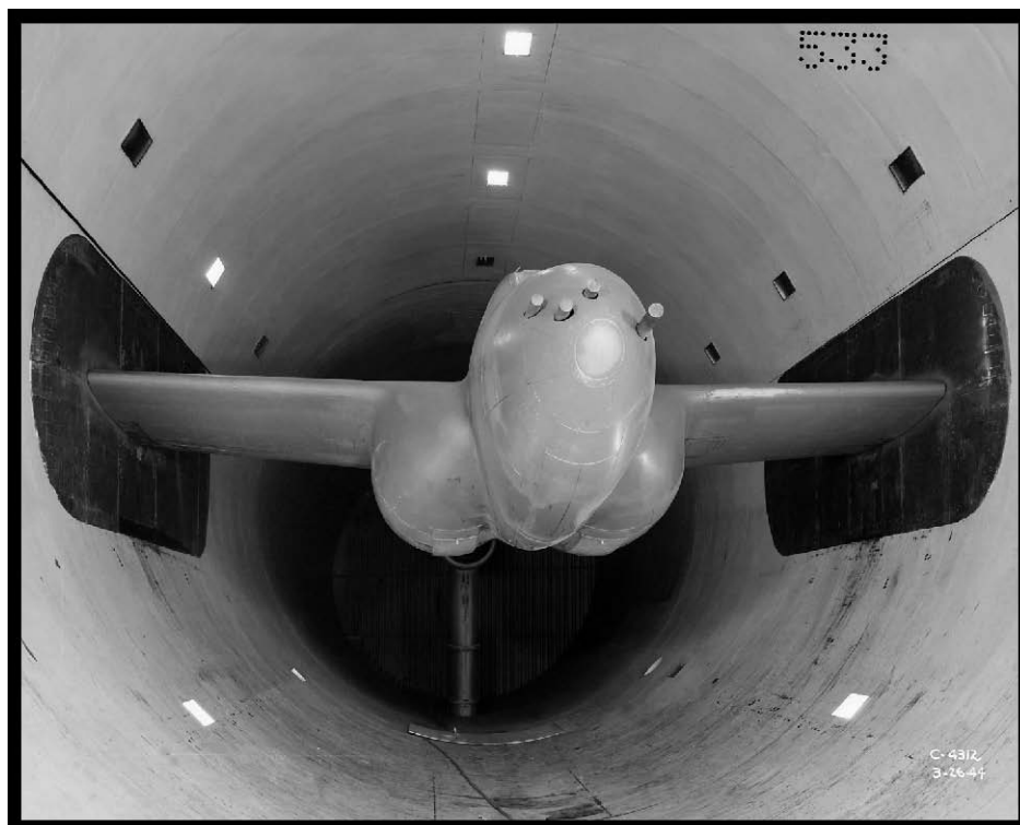
Figure 109.—Although not anticipated initially, the test section was large enough to test entire jet aircraft, 1944 (OH_Cuyahoga_Altitude-Wind-Tunnel_110).
