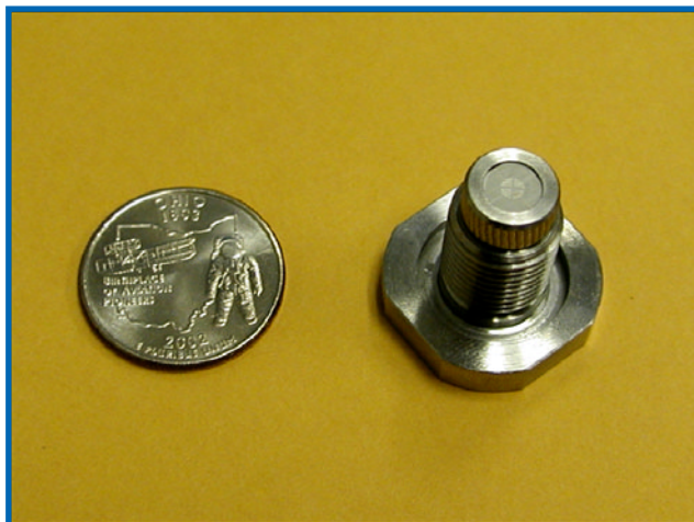
Figure 2.—The single-sided Wheatstone bridge heat flux sensor in a mounting bolt.
