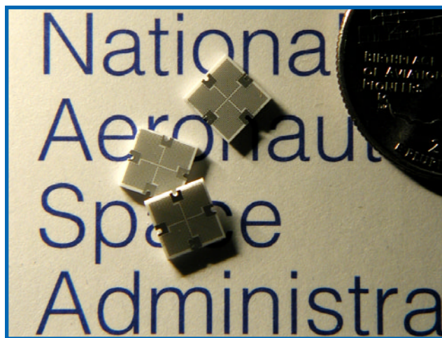
Figure 5.—Double-sided Wheatstone bridge heat flux sensor elements.
