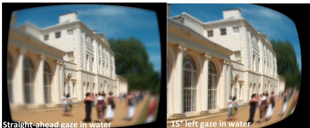
Modelled xEMU Visor Distortions. From Brunstetter et al., Vision/Optical Challenges of NBL Ops (2025)
