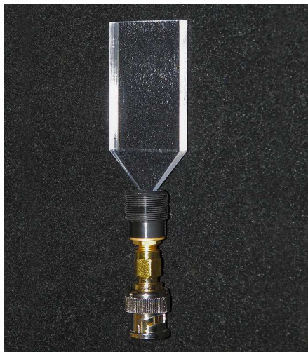
NASA Glenn's Low-Power Charged Particle Detector is compact and robust.
