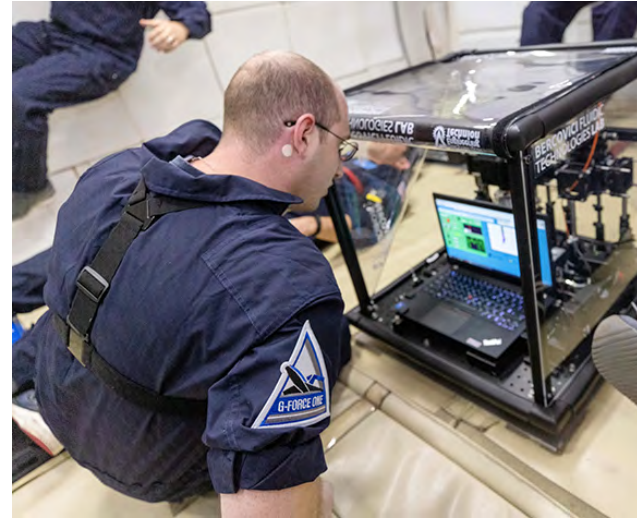
Multiple rounds of parabolic flight testing enabled Edward Balaban of NASA's Ames Research Center to test various liquids, geometries, and deployment mechanisms to optimize future development of the fluidic telescope. Credits: Zero Gravity Corp./Steve Boxall
