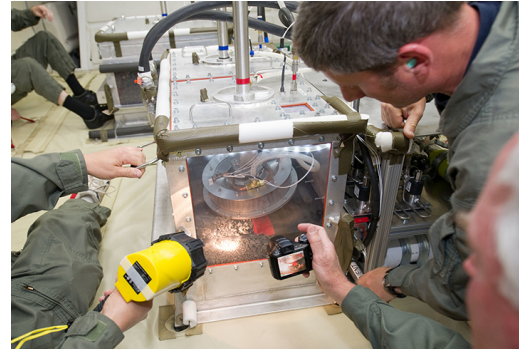
Evaluating OSIRIS-REx sampling system in microgravity via Flight Opportunities in 2012. Credits: NASA/James Blair
