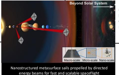
SOA: Conventional fueled propulsion methods are limited by the rocket equation and solar sails are limited by low-intensity sunlight; optical actuation by lasers is primarily limited to nano/microscale particles and objects.
