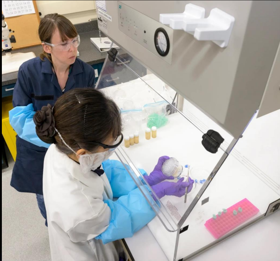
After hardware is fabricated, & sterilized, it is loaded with organism & growth media.
