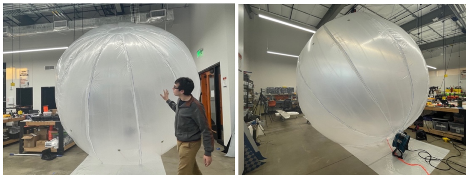
Figure 52 Initial 1.0 mil thick 1/20 th scale model Pluto EAD
