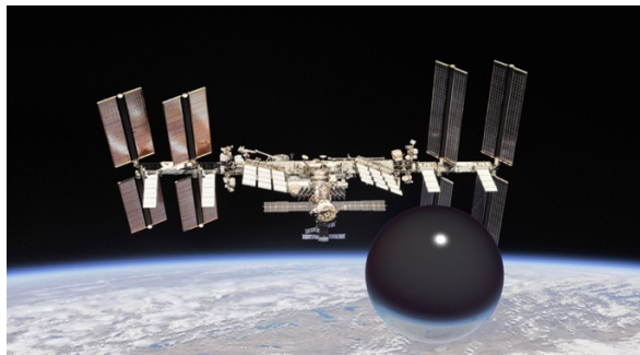
Figure 31. Atmospheric Density Monitoring System just released and deployed from ISS.
