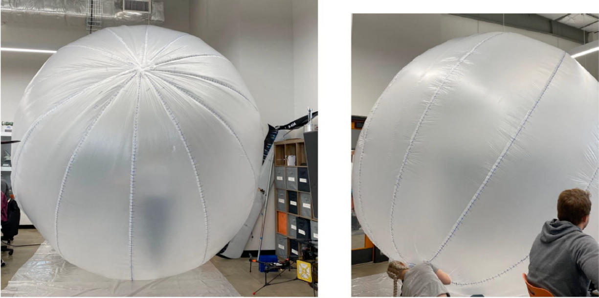
Figure 53 0.3 mil thick 1/20 th scale model Pluto EAD
