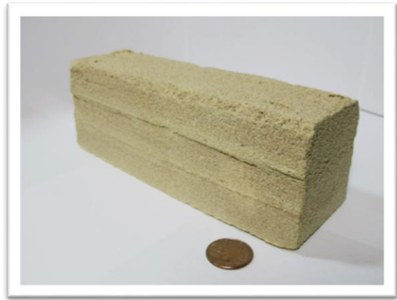
Figure 22: Three layers extrusion sample
