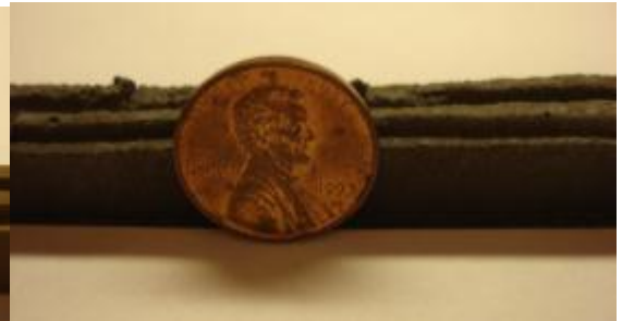
Figure 27: Single layer of lunar sulfur concrete
