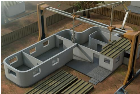
Figure 1: Gantry robot structure for contour crafting
