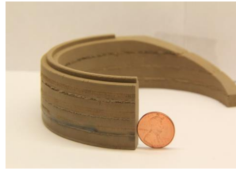
Figure 10. Sulfur concrete part made with Contour Crafting.
