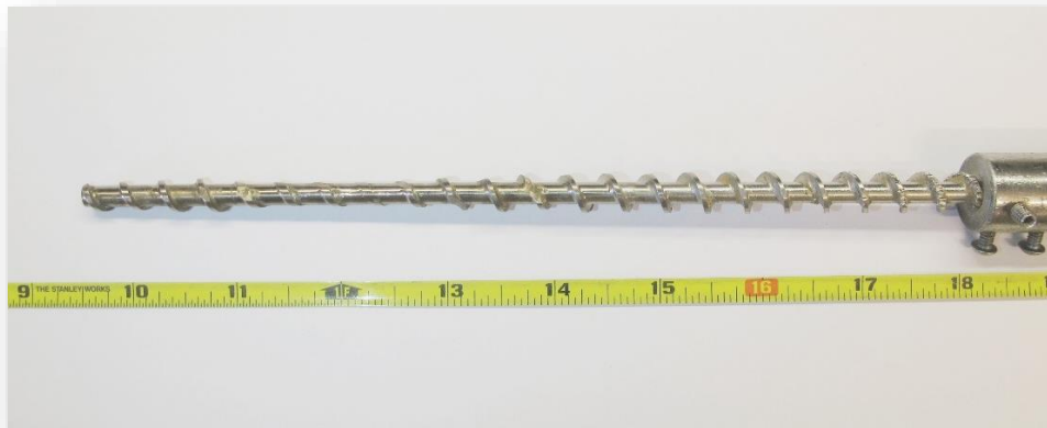
Figure 17: Auger worn-out during experiment
