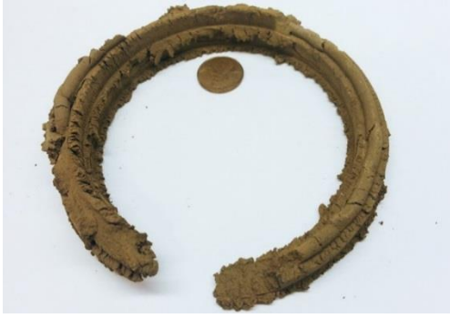
Figure 15: Extruded sample with crack on surface
