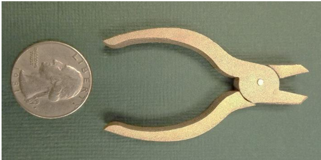
Figure 9. Inter-locking metallic parts made with SSS
