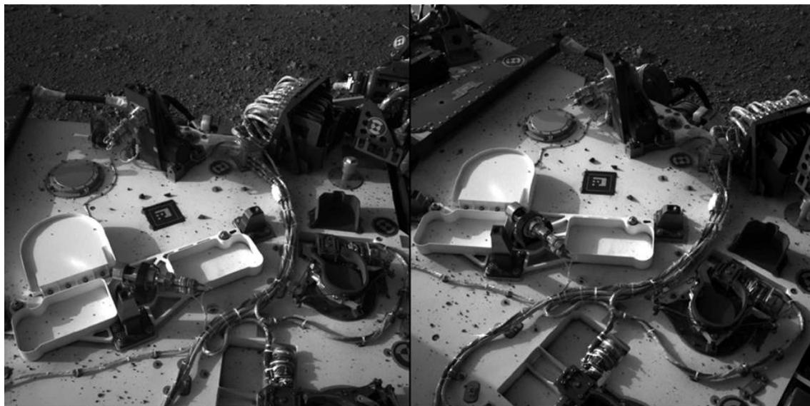
Figure 13. The view through Curiosity's left (A) and right (A) Navcams, looking down on the deck of the rover just after touchdown shows martian soil strewn all over the payload platform. The energy imparted by energetically scattered debris was sufficient to damage an exposed anemometer on the rover.[Credit: NASA/JPL-Caltech]
