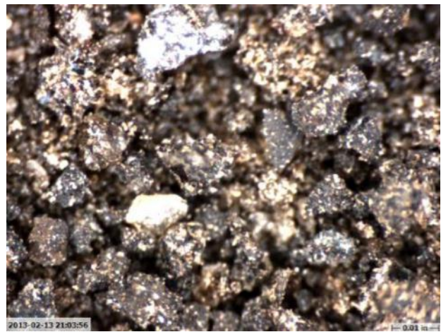
Figure 31: Sifted JSC-1A Lunar regolith simulant (x92)
