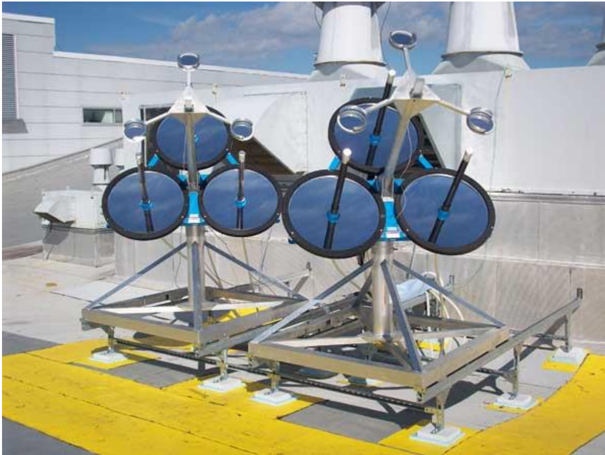
Figure 28. Optical waveguide solar energy concentrators could be used to pipe energy directly to the end effector of the CC or SIS systems. Since the construction system is meant to operate in
