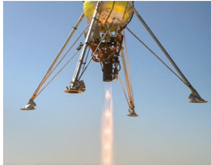
PlanetVac was flight tested in the "feet" of a vertical takeoff and vertical landing vehicle. Credits: Astrobotic
