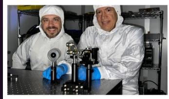
Tyler Groff (left) and John Hagopian tright) display a carbon nanotube patterned apodizer mirror used in the NASA Goddard Space Flight Center coronagraph test bed. Credit: Advance Nanophotonics/John Hagopian, LLC
