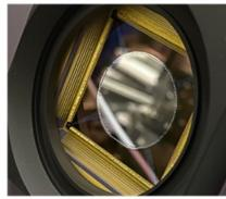
A Boston Micromachines Corporation (BMC) 2k DM with 2040 actuators on a 400-µm pitch. Image credit: Eduardo Bendek
