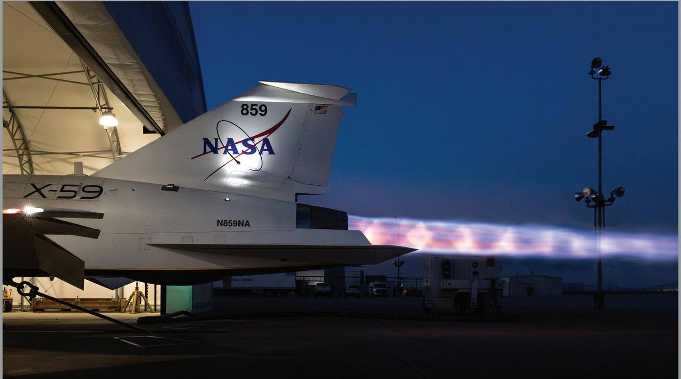
NASA's X-59 lights up the night sky with its unique Mach diamonds, also known as shock diamonds, during maximum afterburner testing at Lockheed Martin Skunk Works in Palmdale, California. The test demonstrated the engine's ability to generate the thrust required for supersonic flight, advancing NASA's Quesst mission. Lockheed Martin/Gary Tice
