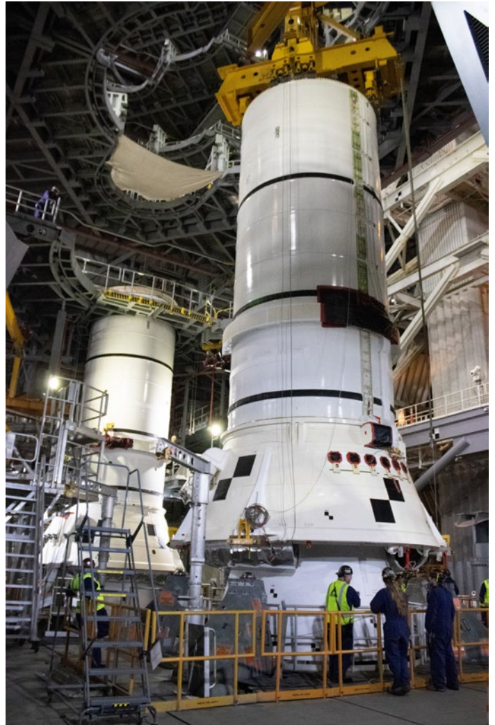
The aft assemblies of the solid rocket boosters for NASA's SLS (Space Launch System) rocket that will launch the Artemis II mission are on mobile launcher 1 at NASA's Kennedy Space Center in Florida.
