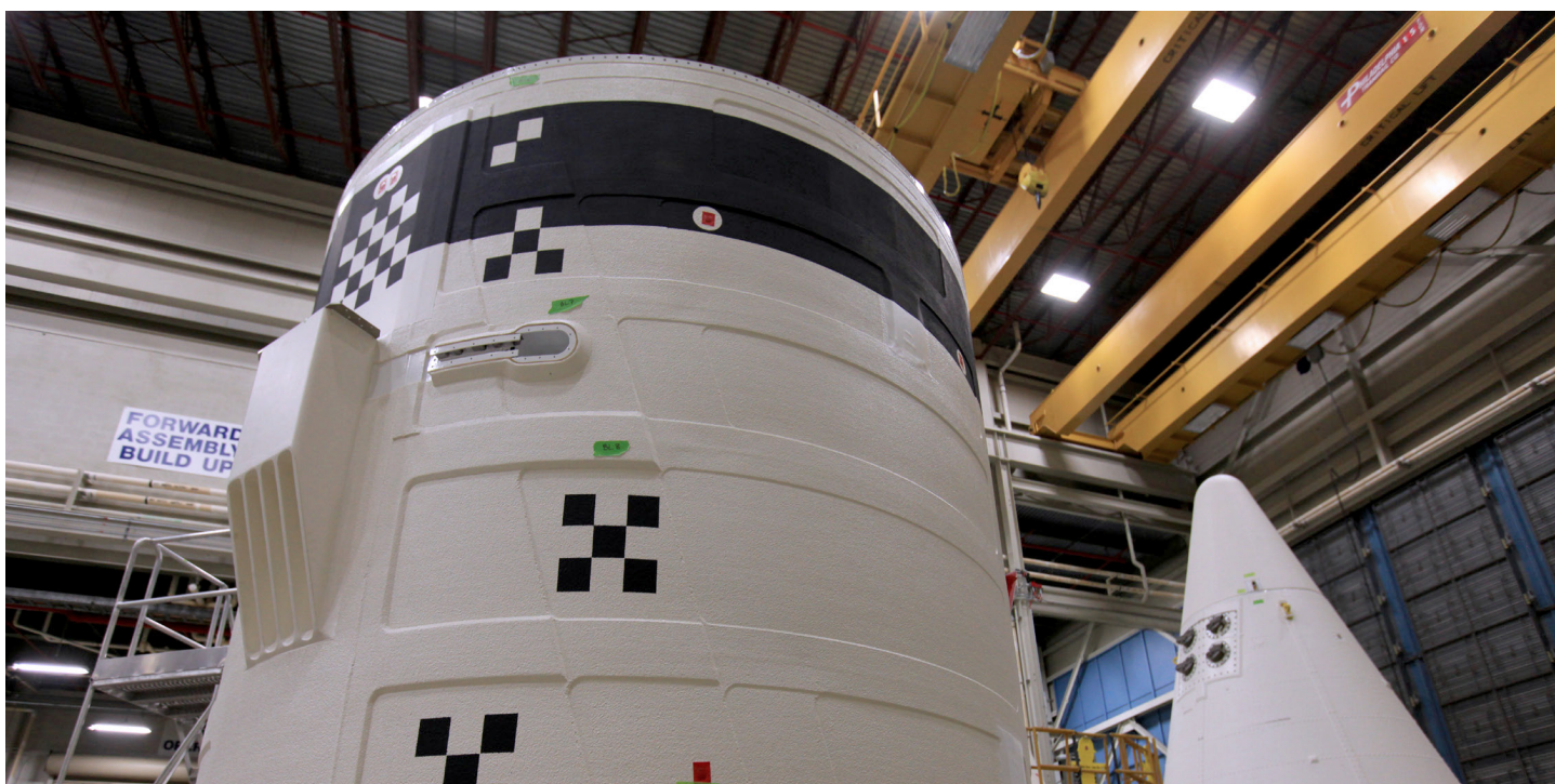
Once mated, the forward skirt (front) and the nose cap (back) form the forward assembly, or top section, of the SLS solid rocket boosters.
