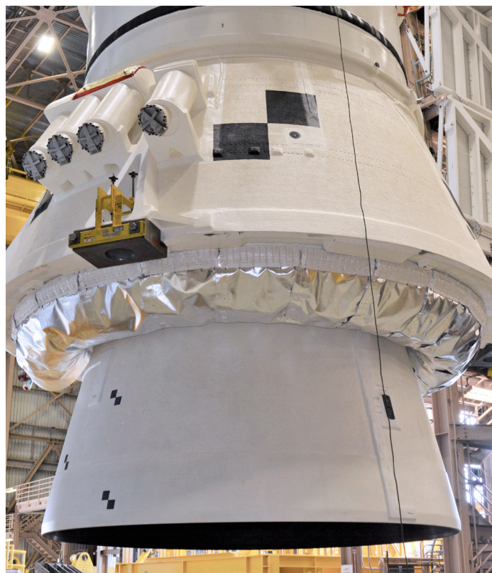
At the Booster Fabrication Facility (BFF), a completed aft skirt assembly can be seen with its four booster separation motors.
