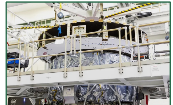
European Service Module 3 joined with Crew Module Adapter
