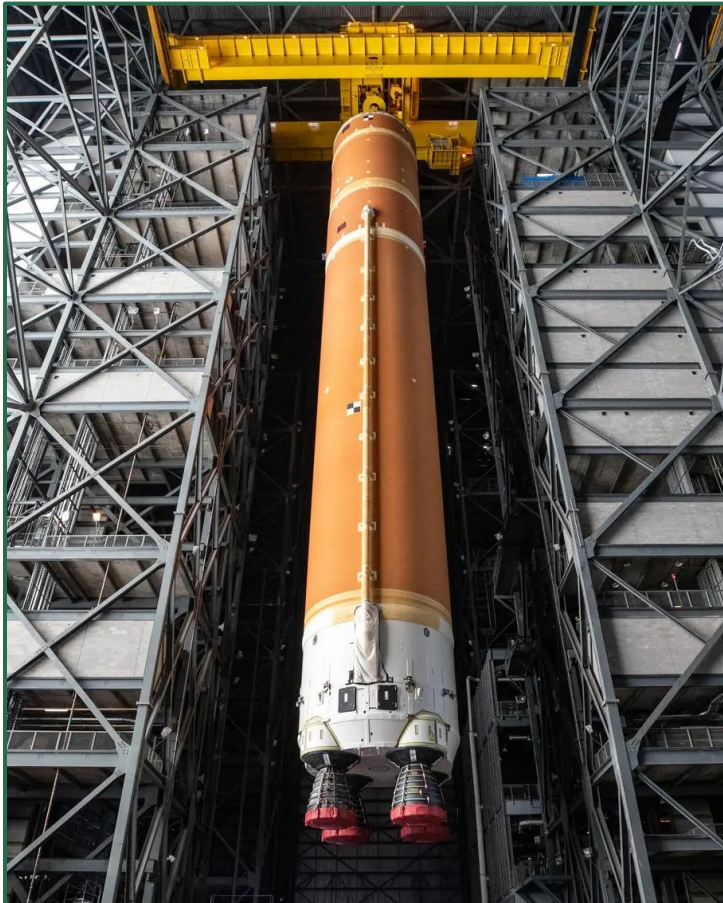
Artemis II core stage is 'hard down' and fully supported by the structure in High Bay 2 in the Vehicle Assembly Building on Dec. 12, 2024
