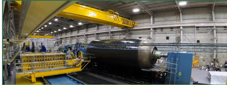
Trial Booster Obsolesces and Life Extension (BOLE) for Artemis 9 composite case winding
