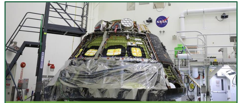
Artemis I Orion crew module, now the Orion Environmental Test Article, returned from Glenn after 11-month testing campaign to undergo propulsion functional testing
