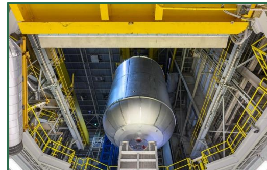
Core stage liquid oxygen tank completed hydrostatic proof testing
