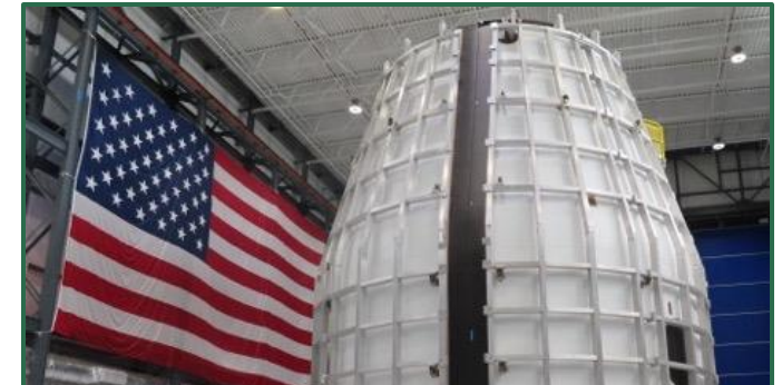
All four universal stage adapter structural qualification article panels are aligned and loaded on Vertical Assembly Tool
