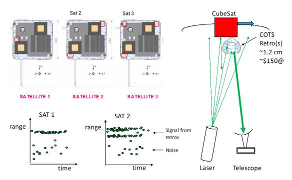
Figure 12.6: Corner Cube Reflectors. Credit: The Aerospace Corporation.
