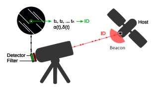
Figure 12.3: ELROI Optical Detection System. Credit: Los Alamos National Laboratory.
