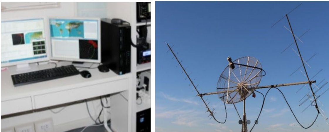
Figure 11.21: (left) GAUSS ground station hardware, transceiver and (right) tracking antenna. Credit: GAUSS Srl.
