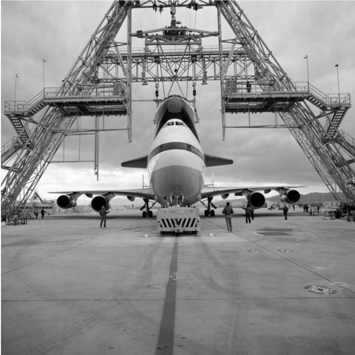
Figure 10. The Orbiter Endeavour being mated to NASA 911 in the Orbiter Lifting Frame at Palmdale for her initial delivery to Kennedy Space Center, May 1, 1991.
