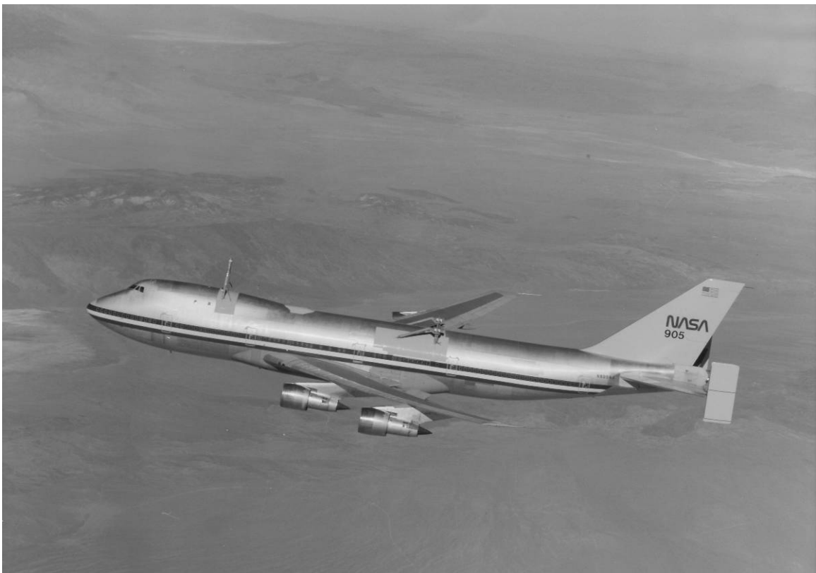
Figure 2. View of the NASA 905 following modifications to become the first SCA, December 23, 1976. Source: NASA DFRC, ECN-6356.
