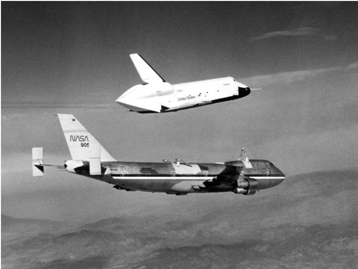
Figure 3. View of the orbiter Enterprise detaching from NASA 905 during one of the Approach and Landing Test Program free flight tests, September 26, 1977.
