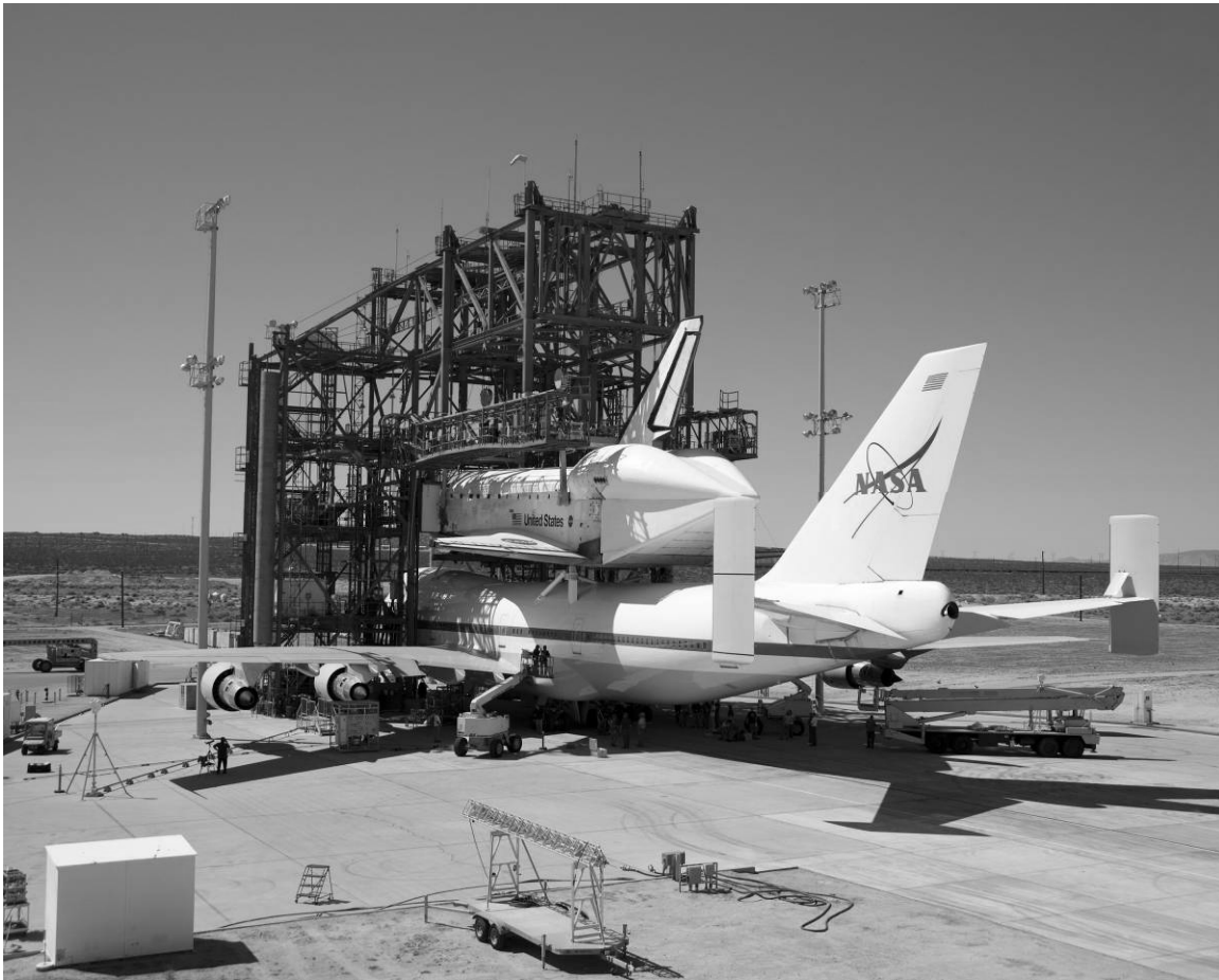
Figure 11. View of the orbiter Discovery being attached to NASA 911 for the final post-mission ferry flight of the Space Shuttle Program, September 18, 2009.
