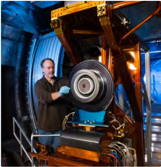
Top: NASA engineer Dr. Peter Peterson, prepares a high-power Hall thruster for ground testing in a vacuum chamber. Credit: NASA
