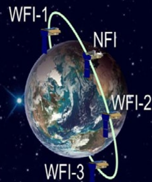
Sun-synchronous orbit; 6:00AM local time ascending node
