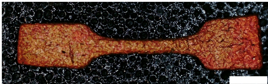
Copper dogbone CAL-HIAM part. Scale bar: 1 mm (Left). Initial batch of dogbones fully processed (Right).
